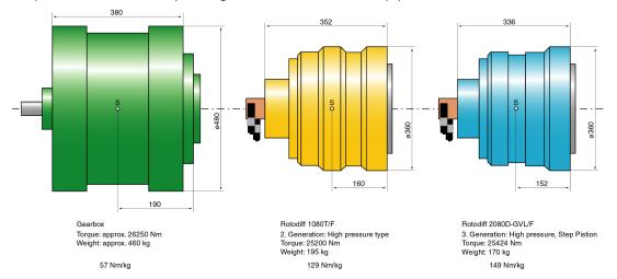
This latest "STEP PISTON" development enables Viscotherm to be technically superior and price competitive at the same time, due to the 50% enhanced torque capacity on equal Rotodiff sizes, additionally the new step piston design has less moving parts, therefore increased lifetime and reduced maintenance and operating costs are further advantages.
