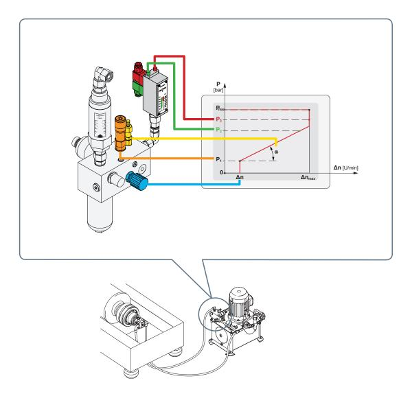
P.... Pressure cut off point (pressure relief valve)
