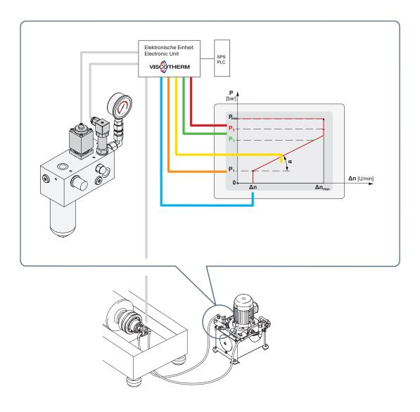
Pressure cut off point (pressure relief valve)
